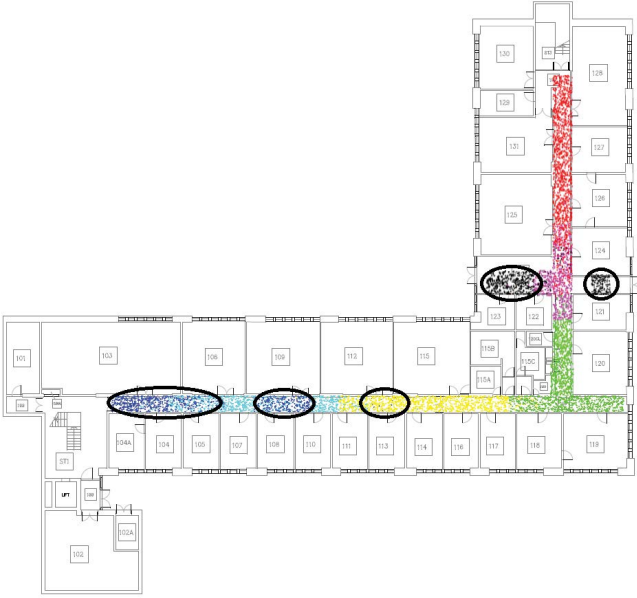
Figure 1: Islands with similar WLAN signals visualised on 2-D floor plan of our office.
