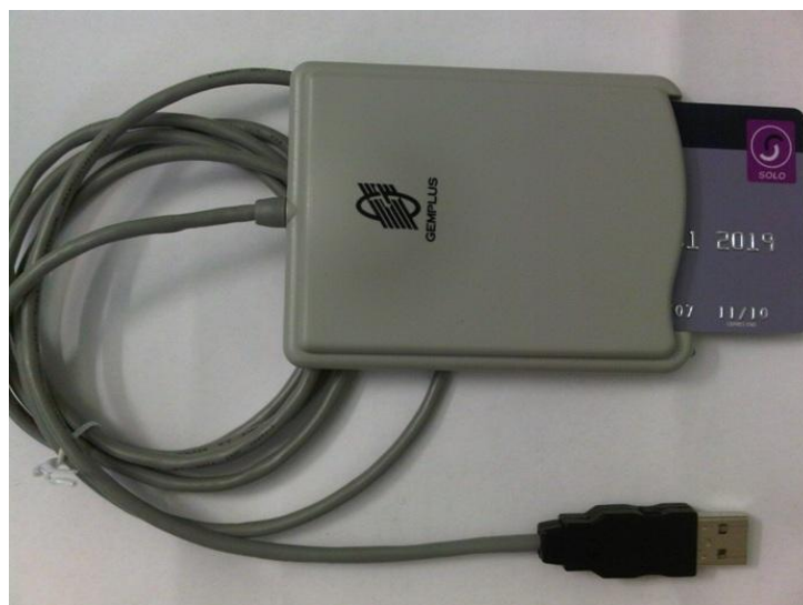
Figure 3: Smart card reader used in this project
